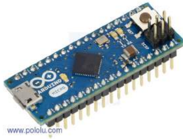
Figure 6: A picture of the Arduino Micro micro-controller which is the processing unit of the strut.
