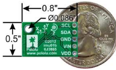
Figure 7: A photograph of the Inertial Measurement Unit that was chosen to be used in the final design.
