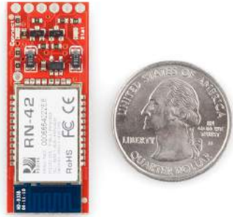
Figure 9: A photograph of the BlueSMiRF unit that was chosen to be used in the final design.
