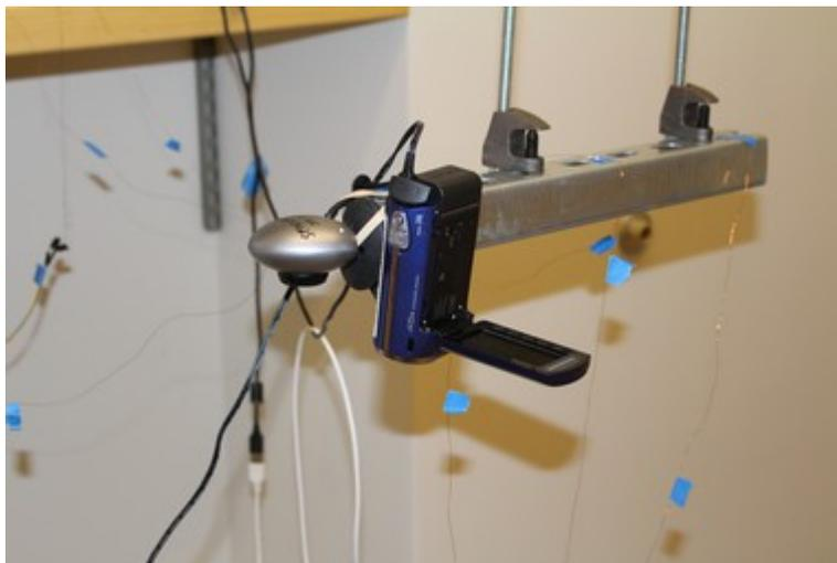
*Image 2: The camera mounted above the tensegrity. The camera is used to capture the motion of the robot.*
