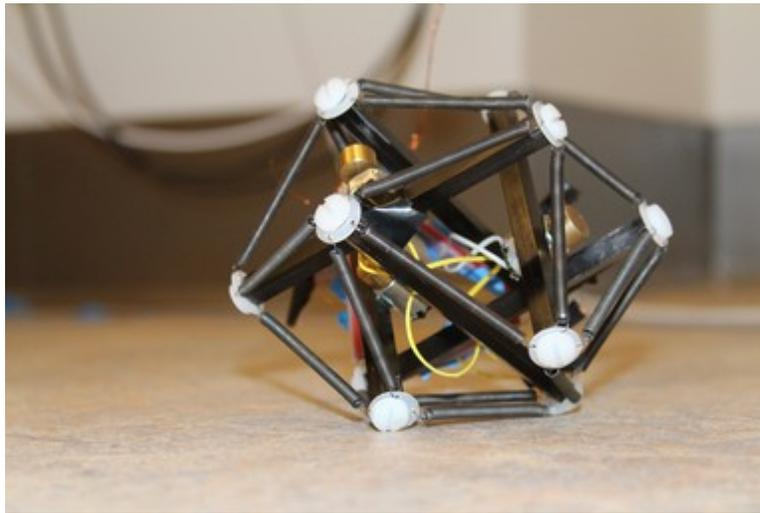
*Image 1: A picture of a 6 bar tensegrity.*
