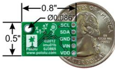
Figure 6: A photograph of the Inertial Measurement Unit that was chosen to be used in the final design.
