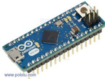
Figure 5: A picture of the Arduino Micro micro-controller which is the processing unit of the strut.
